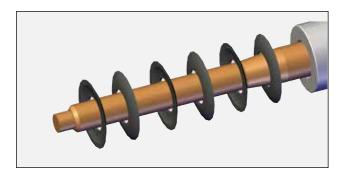
11. Install rear nut. Install jam nuts finger tight.
