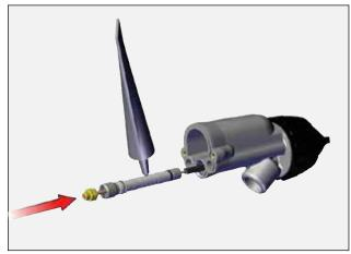
2. Tighten packing using wrench. Pull back and forth on the needle shaft till a slight amount of drag is felt.
