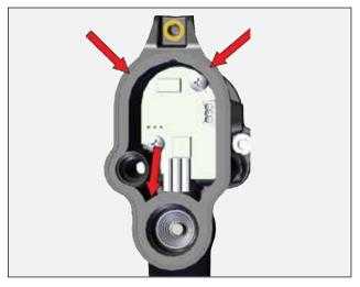
8. Push rear cover assembly into handle and tighten cartridge.
