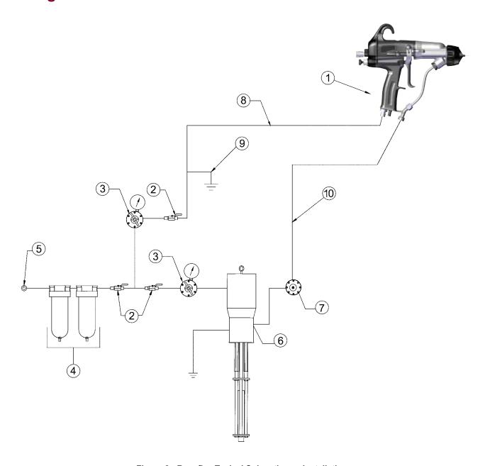
Figure 2: Ransflex Typical Solventborne Installation
