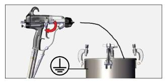
4. Release trigger stop material flow.
