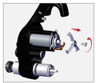
3. Remove motor assembly by pulling out on 3 arms, pull motor out.
