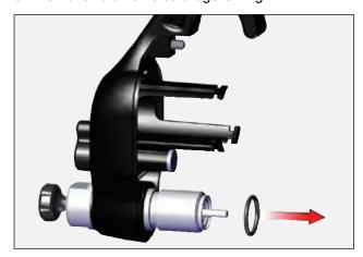
6. Push on edges to remove fluid valve cartridge.
