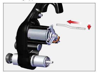
6. Install fluid valve cartridge.
