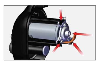
3. Install cartridge then o-ring (if removed).
