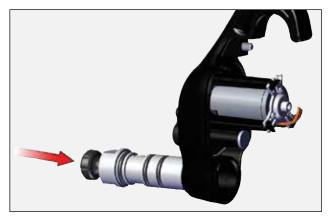
7. Install gasket and re-connect motor connector to handle harness connector.
