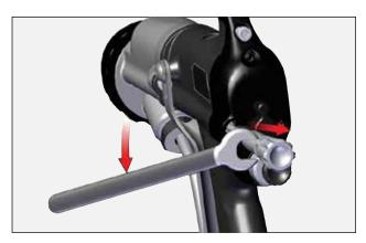
3. Remove rear cover and cartridge with 15mm wrench.
