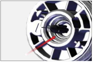
Install fluid nozzle using 80353-00 wrench.
