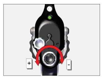
15. Adjust compensation valve with small driver.
