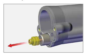
4. Remove jam nuts using 10mm wrench.
