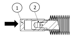
Screw Item No. 2 (assembly spigot) onto the piston shaft
